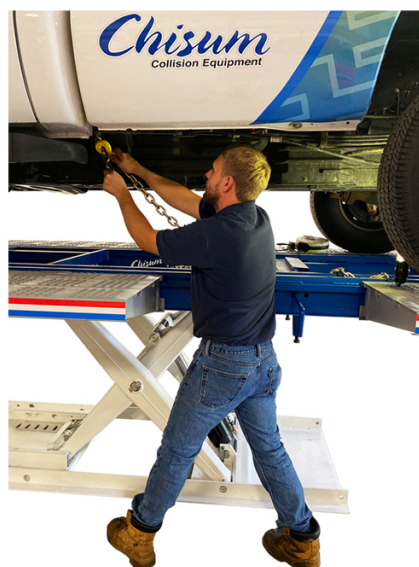
Removable treadways allow access for inspection and chaining vehicles
