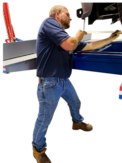
Removable treadways combined with adjustable work height allow technicians to work ergonomically and efficiently especially when using a tram gauge to take basic measurements
